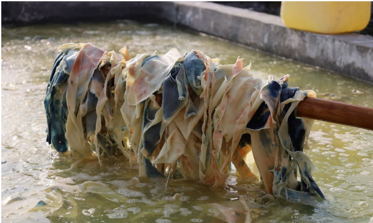
Pieces of fabric being bleached at a textile recycling unit in Faisalabad
