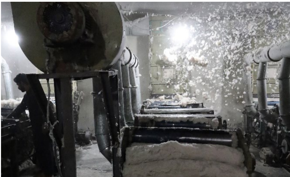
An operating shredding machine in a textile recycling unit in Faisalabad
